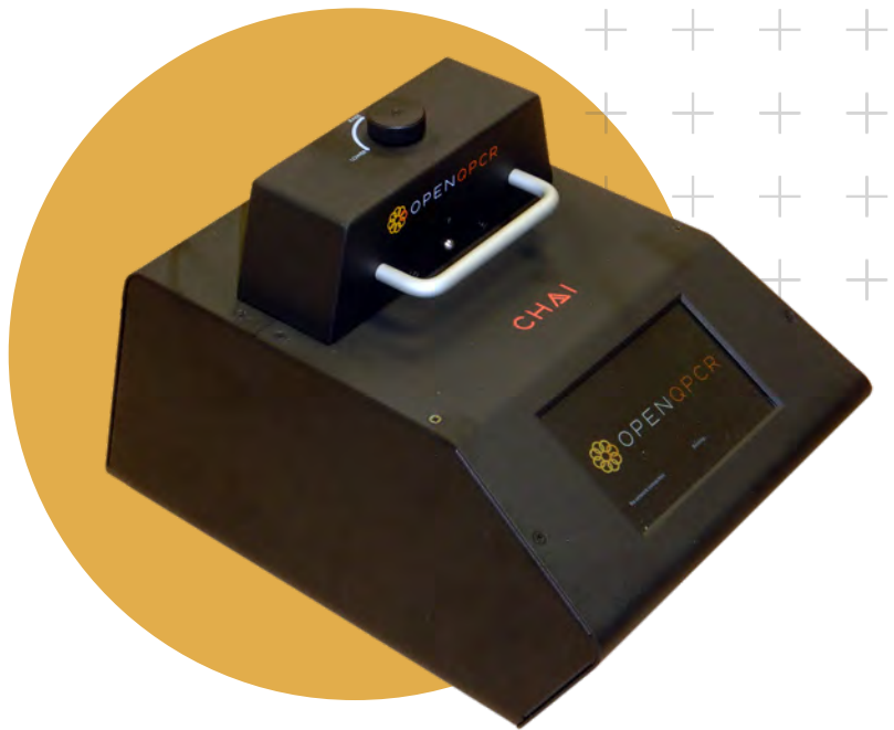
Devices that perform eDNA analysis are now portable and affordable. Shown here is the tabletop device used by my team.
