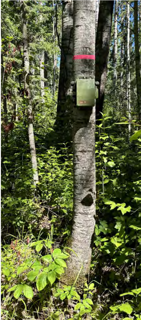
An autonomous recording unit (ARU) used for monitoring songbirds associated with linear features in the boreal forest. THARINDU KALUKAPUGE
